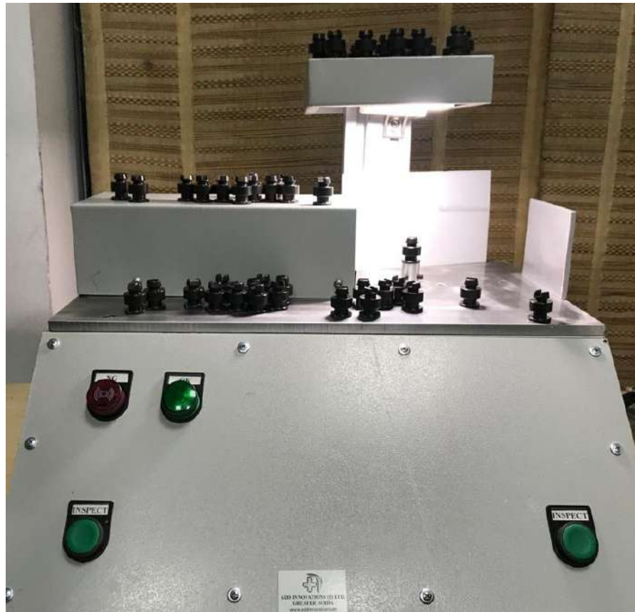
Add Innovations hydraulic brake inspection system at Tasa Automotive plant in Haryana
