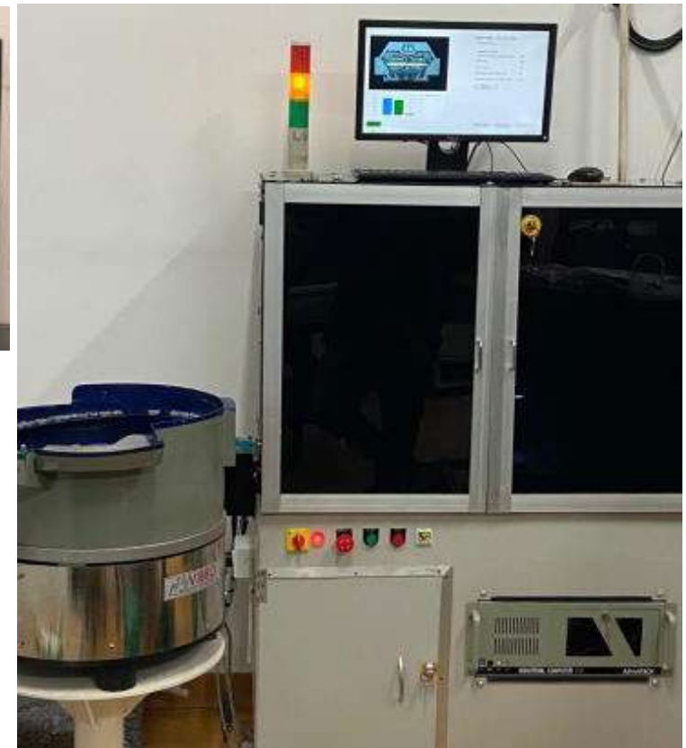
Add Innovations Vision system for high speed connector inspection at Wago factory, Noida. See system in action here (YouTube)
