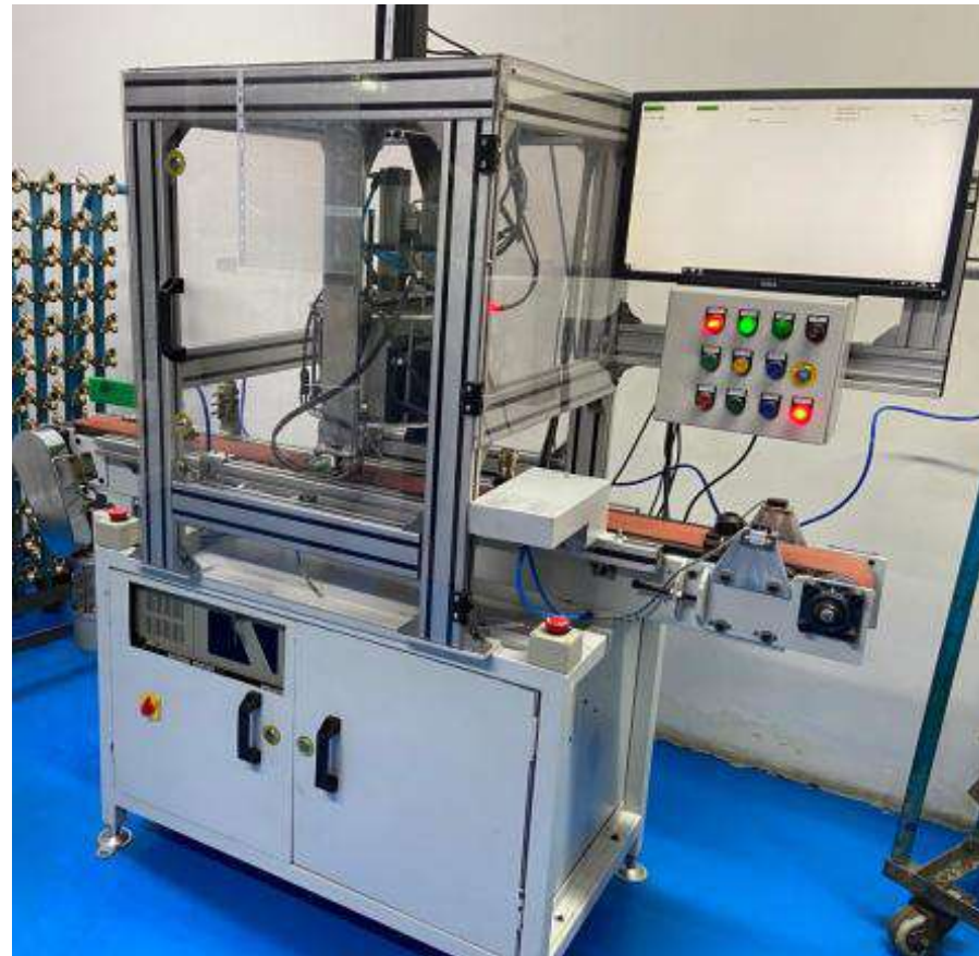
Add Innovations Vision system for surface defect inspection at Jaquar plant, Haryana. See system in action here (YouTube)
