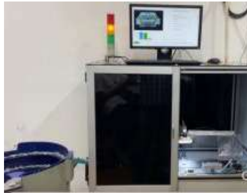
Add Innovations Vision system for high speed connector inspection at Wago factory, Noida. See system in action here (YouTube)
