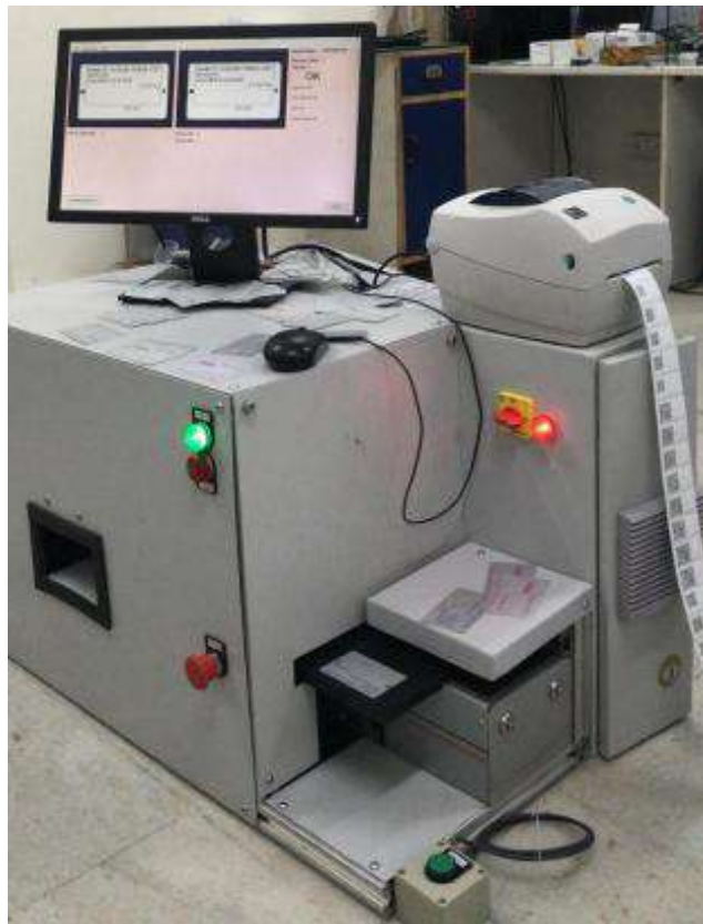
Add Innovations Print Content and Quality Inspection System being used on Maruti Suzuki Vehicle Identification Plates
